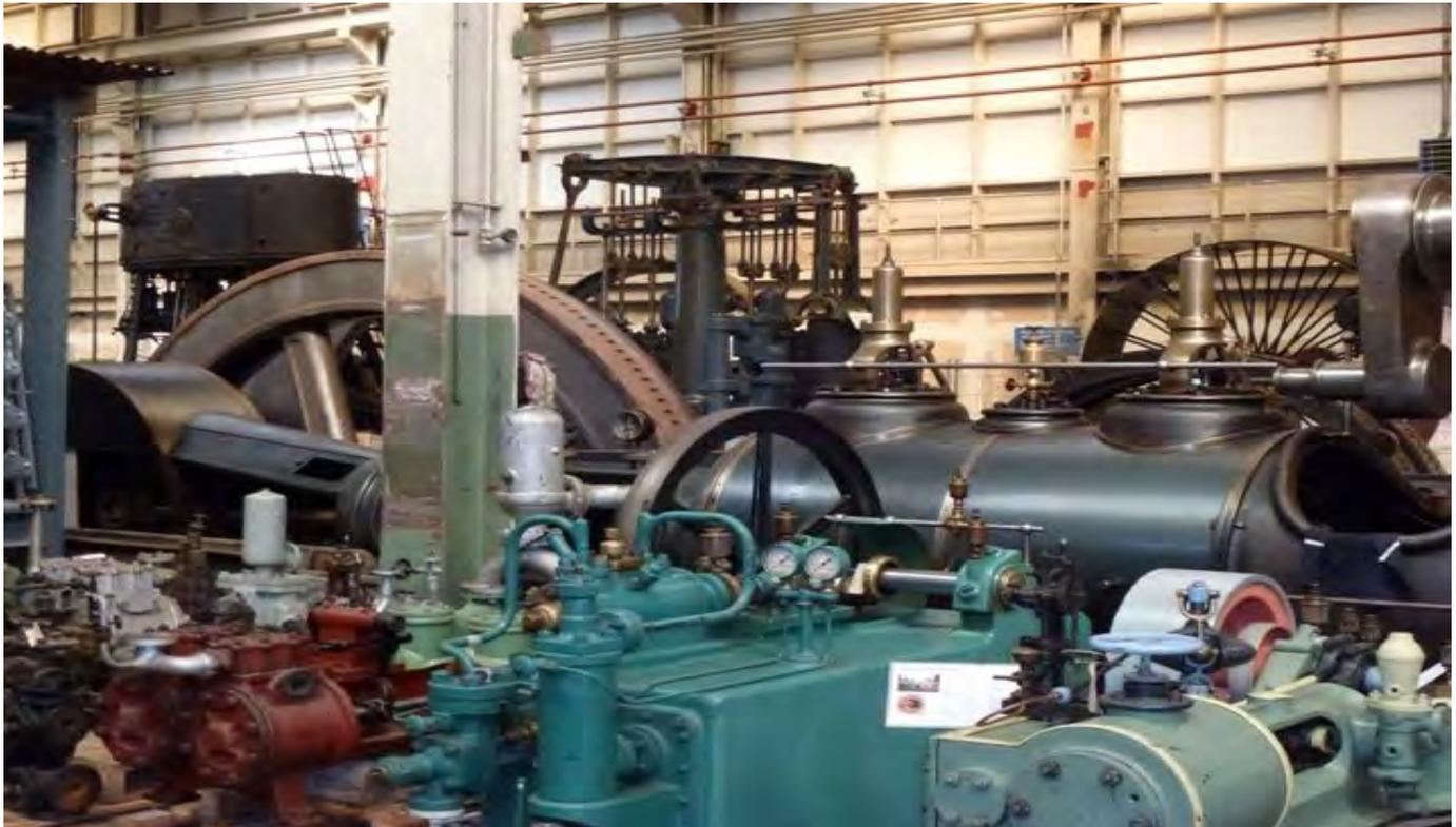
The Steam Centre Winterthur. Left in the back you can see the three-cylinder Sulzer steam engine shown at the Paris World Exhibition of 1889 and next to it stands the 1859 German beam engine. In the middle is a big and typical Sulzer engine with valve control. In the foreground are smaller parts of the collection.
